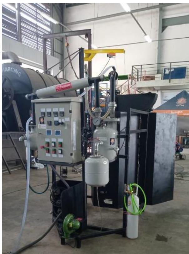
The special equipment prepared for the first pyrolysis of insecticide-treated mosquito nets (Carnevale et al. , 2025).
