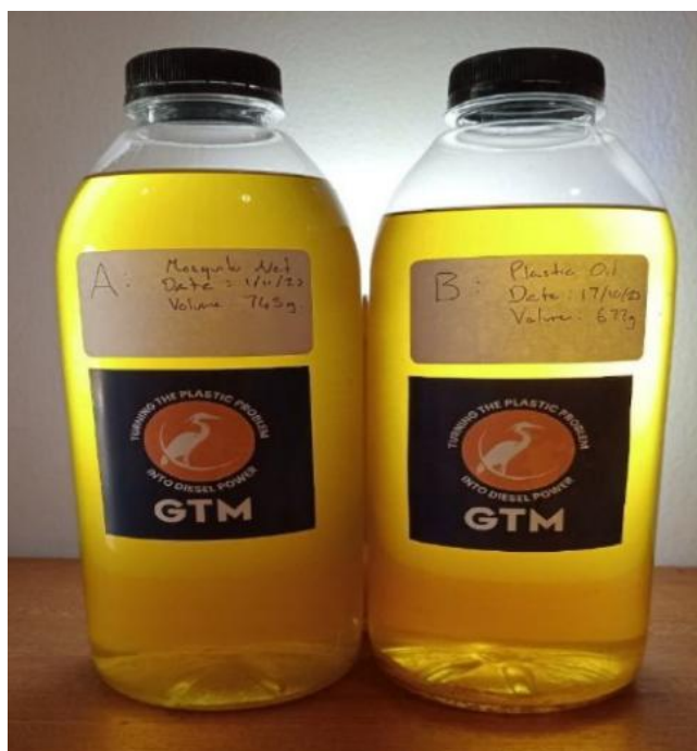
Sample of oil obtained by pyrolysis of nets (left) and domestic plastic waste (right).
